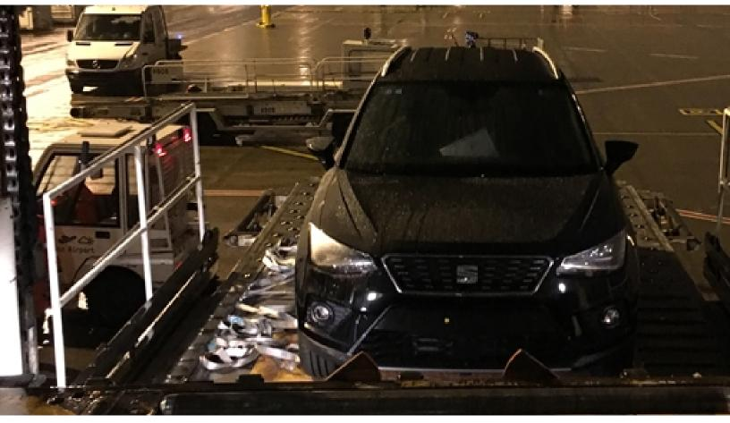
Caption: The Seat Arona, which due to its vehicle dimensions cannot be loaded on pallets in the lower deck of an Airbus A330, was loaded and unloaded on the Eurowings flight using the roll-in procedure.
